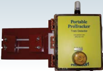
Portable Train Detector, placed inside or outside the track.
