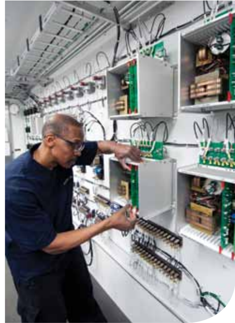
Genrakode™ II Modules being installed in a housing unit at the Rochester, NY facility
