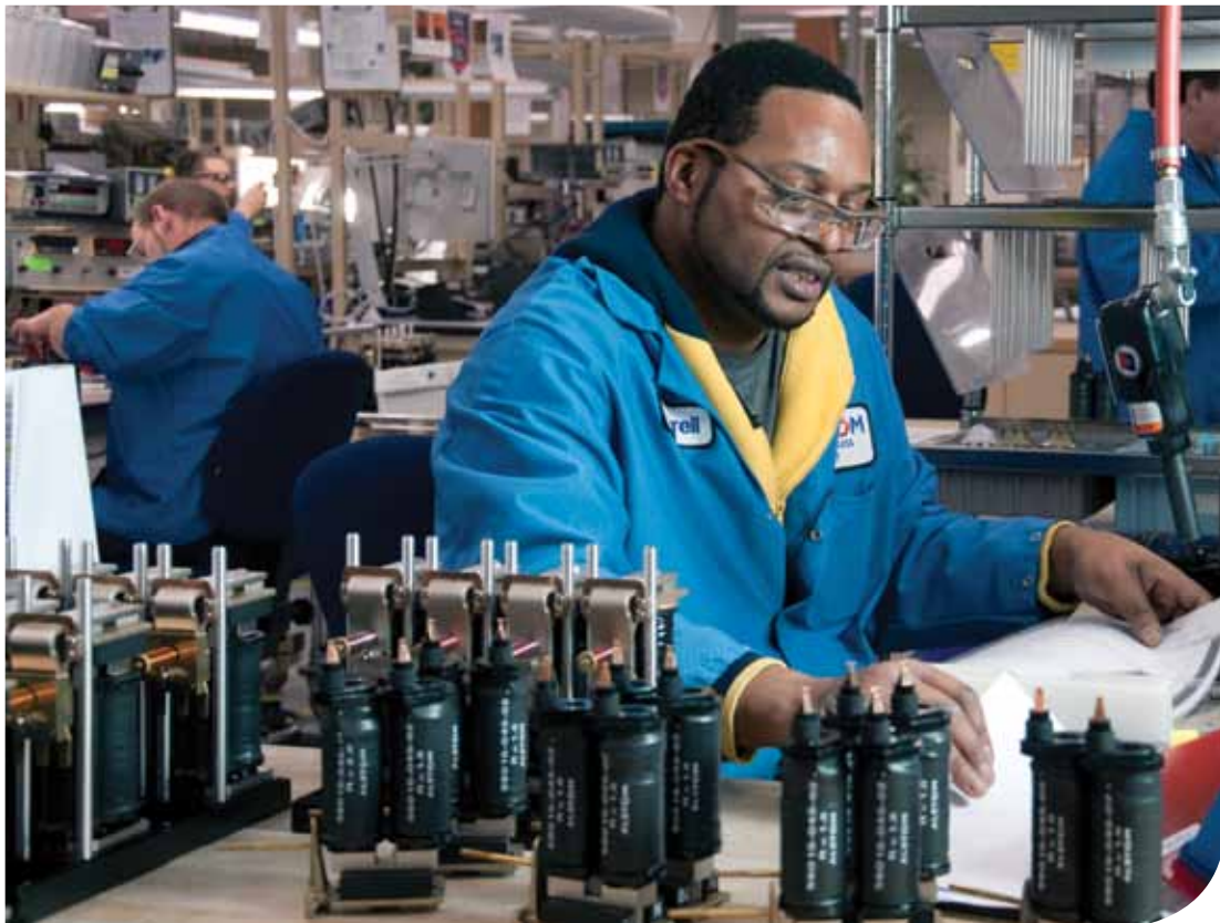
Type B Relay Being Assembled at the Rochester, NY Facility
