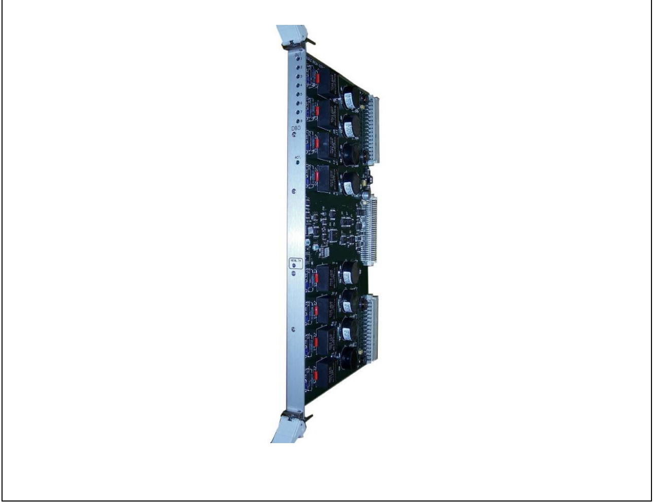
Figure 4–5. Double Break Output Board
