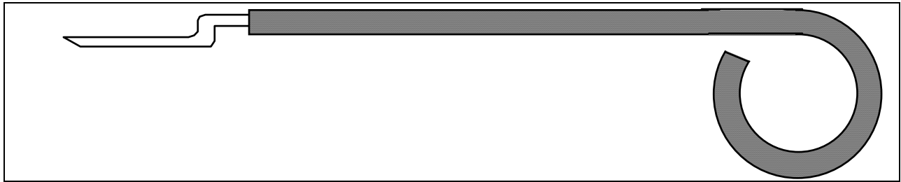
Figure 4-1. Extractor, B Relay Terminal, P/N 59688-000-00
