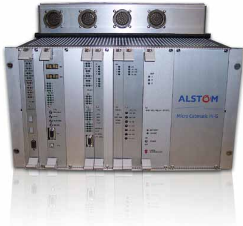
Micro Cabmatic III G capable of providing ATP, ATO, and ATS
